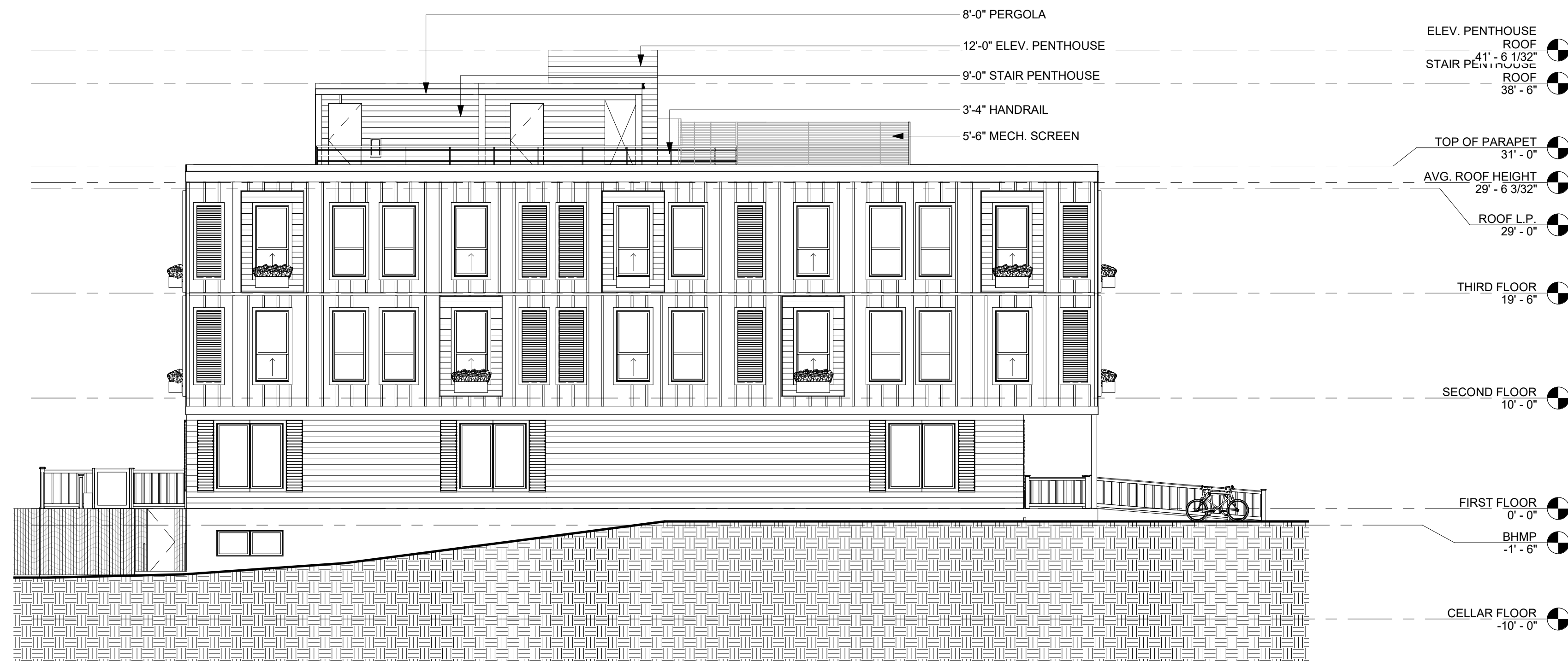
1 SOUTH BUILDING ELEVATION
